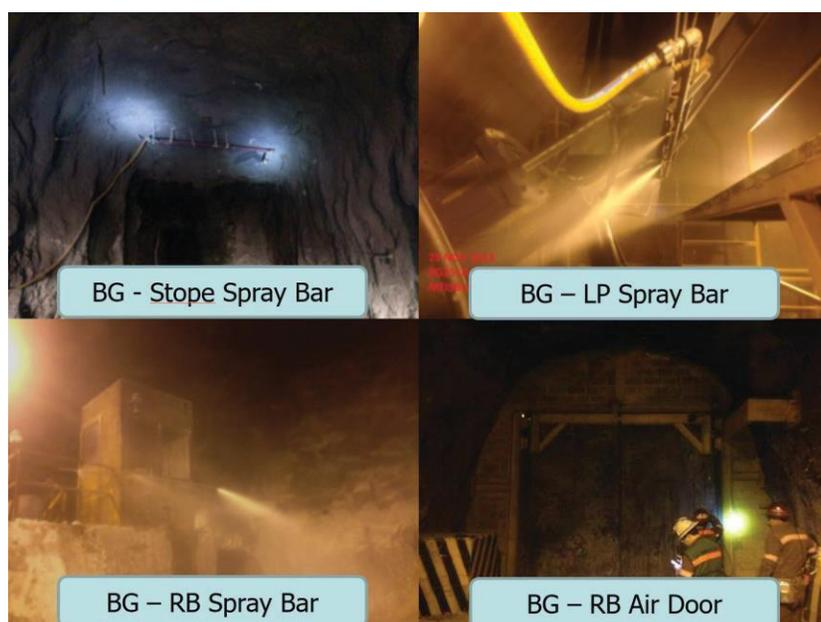
Figure 8: Typical dust controls
