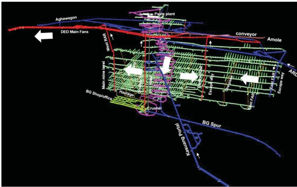
Figure 6: Big Gossan mine ventilation schematic
